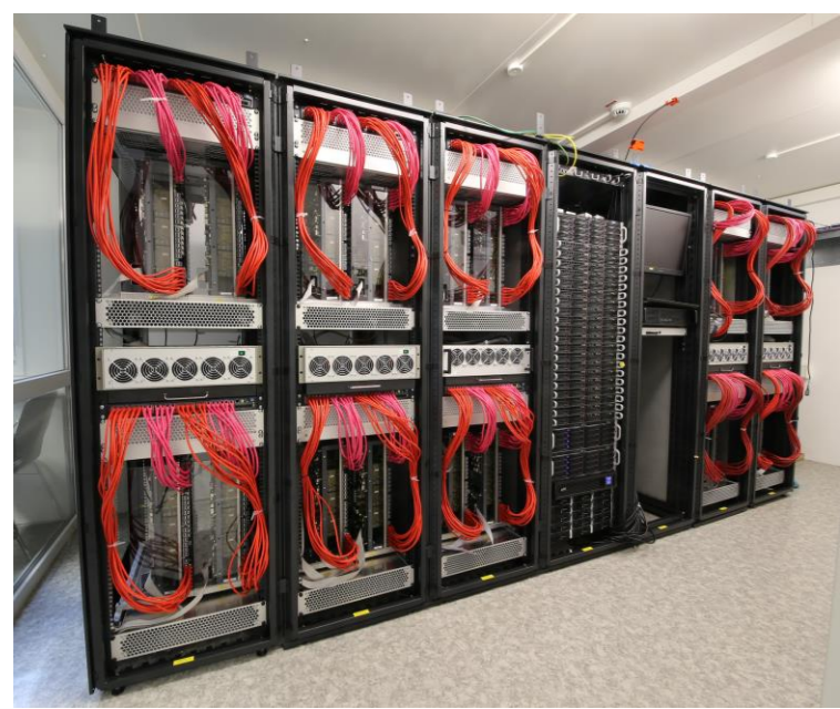
Fig. 1 The BrainScaleS system, consisting of 5 racks with 20 modules and 2 racks with command and control hardware.
