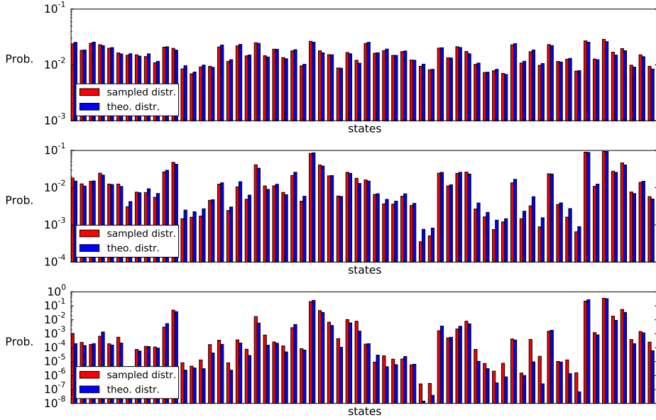
Figure 3.13: Illustration of exemplary distributions that were sampled from. The weights of the noise-generating BMs were scaled with W_0^{\text{noise}} = 1.2 . The sampled distributions shown here were randomly generated with (top) W_0 = 0.6 , (middle) W_0 = 2.4 and (bottom) W_0 = 8.0 . Each pair of bars represents the probability of a network state, once given by the sampled distribution and once by the theoretical target distribution. Note that the probabilities here are shown on a log-scale. For higher weight scale factors, the theoretical target distribution becomes more irregular and the differences between sampled and target distribution increase. However, the network continues to sample consistently from the highest-mass probability modes.
